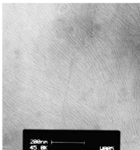
Figure 2. TEM image of copolymer 3C on a carbon-coated copper grid.
